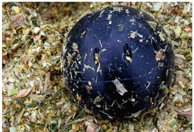
Sensor system for monitoring the ensiling process in biogas production © Fraunhofer IZM
