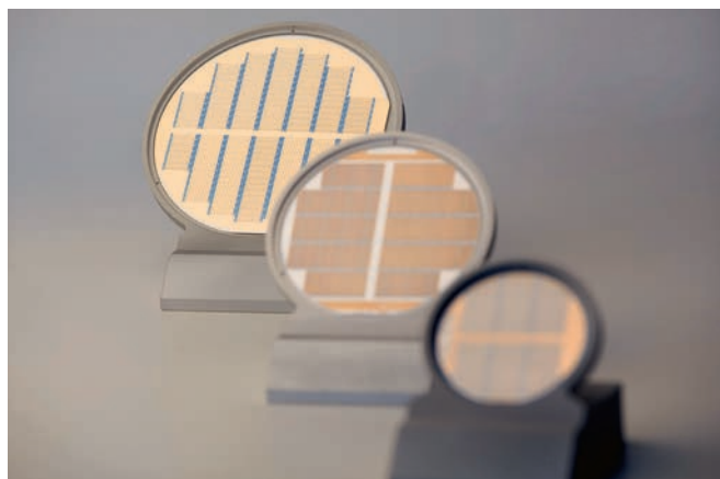
Laser wafers in sizes of 2, 3, and 4 inches © FBH/schurian.com
