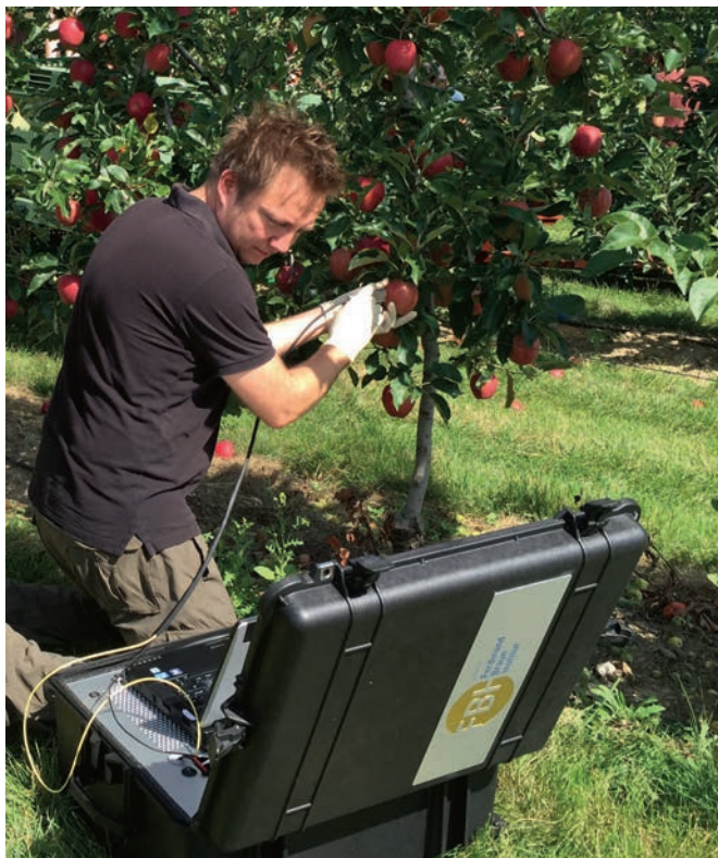
A portable Raman laser system for field use was developed at FBH, seen here in an orchard.
